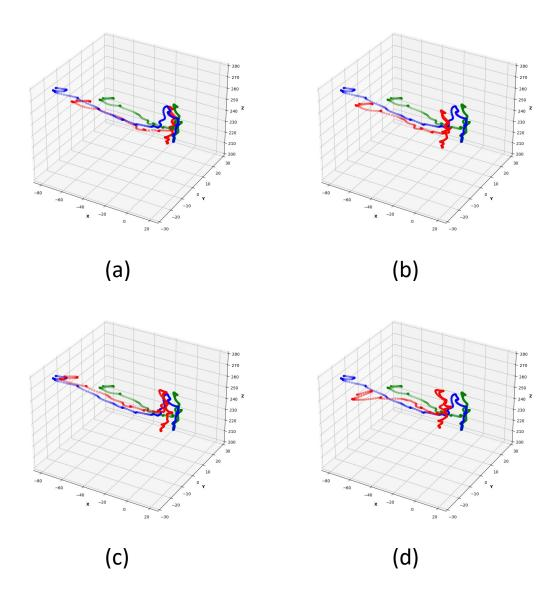
Figure 1. Illustration results of Marker 2 trajectory. (a) The raw data (b) naïve processed data (c) physics-based processed data (d) combination of raw data and physics-based processed data. The (blue) curve denotes ground truth data, the (green) curve denotes input data, and the (red) curve denotes the prediction results.
