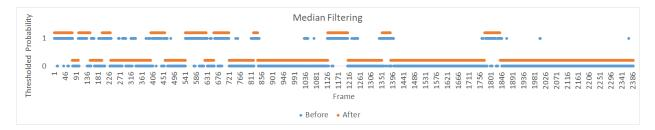
Figure 4. An example of the thresholded probabilities over frame before (blue) and after (orange) median filtering.
