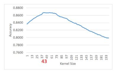
Figure 3. A graph between the kernel size of a median filter and prediction accuracy.
